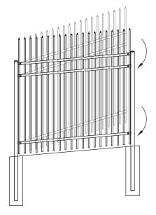
4a - Pivot free end of panel back into brackets & secure; center, if necessary.4b - Tighten all fasteners to ensure permanent grip.
