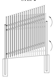
2a - Position panel in brackets & secure with snug fit (finger-tight).2b - Rack free end of panel upward sufficiently to allow space for brackets.
