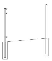
1a - Mount brackets to posts on downhill (downgrade) side only, as shown. Note: Panel must be pre-racked for applicable grade before continuing with Step 2.
